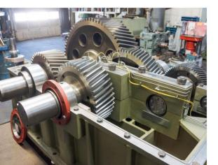
Reassembly of your gearbox is done in our mechanics shop, where great care is taken to keep a clean contaminent free environment. In many cases OEM parts are available, but when they are not, Deca can reverse engineer and manufacture new high quality replacement parts. A final test run of each gearbox is performed to ensure problem free operation, before returning it to our customer.
