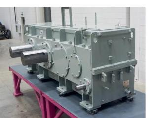
of any worn or damaged components, housing rebuilds if required, reassembly, and final test run before returning it to the customer. Improvements and modifications are available to address bearing life, sealing issues, lubrication, condition monitoring, and premature wear.
